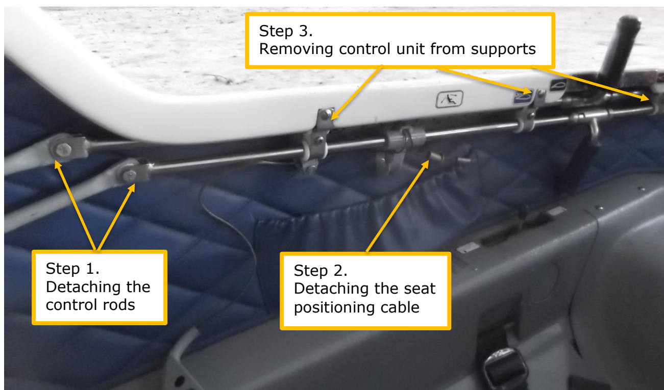
Illustration 2. Removing the flap-air brake control unit
