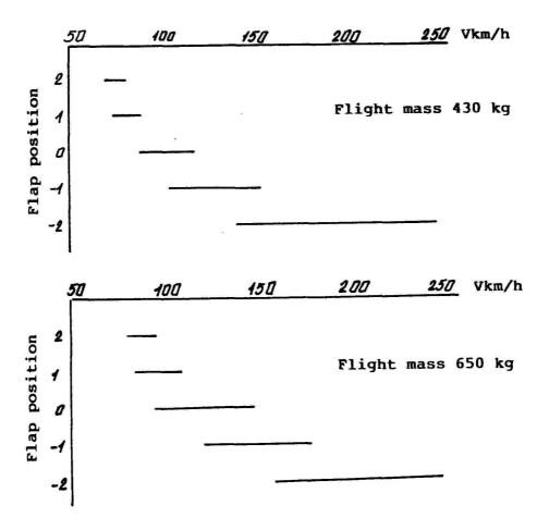
Fig. 4. Dependence of the optimum flap position on the flight speed.
