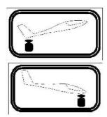
The trim adjustment control knob is located *in the left armrest* and controls the elevator trim select position. See Maintenance Manual Section 2. To set the trim, simply move the adjustment knob to the desired trim position.
