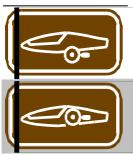
The landing gear is extended and retracted with the gray control handle located in the right hand armrest. Landing gear locked positions are located at either end of the control handle travel. Forward to extend, back to retract. The system is assisted by a nitrogen gas strut. See Maintenance Manual Section 2.
